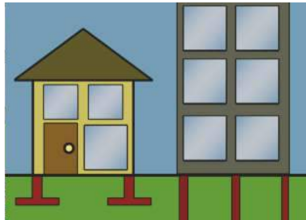
Fig: Shallow foundations of a house versus Deep foundations of a skyscraper
